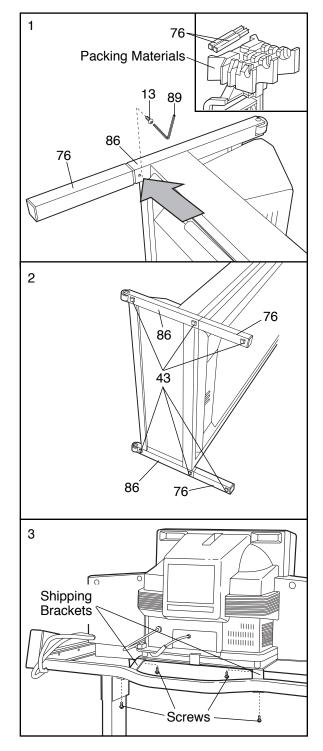
Locate the two shipping brackets on the back of the television. Remove the four indicated screws. Discard the four screws and the shipping brackets.
